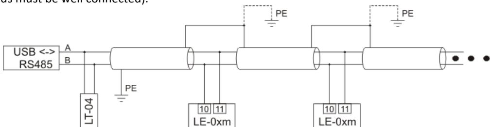
If the energy meters is some ground connection (low impedance), it is recommended to connect the shield of cable to the PE at each meter.
