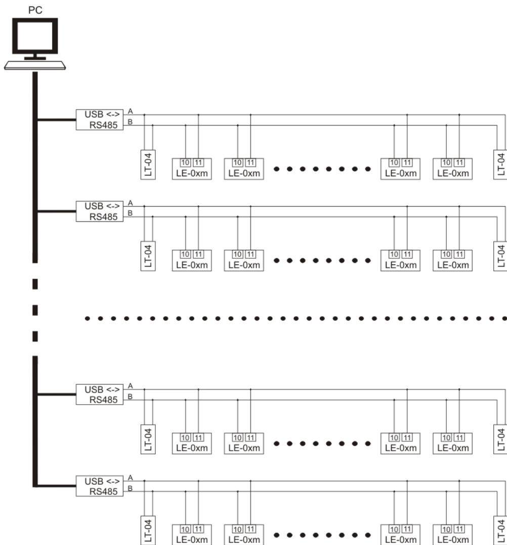
To PC are included USB converters <-> RS485 with the number of planned subnet. At the output of each converter is
